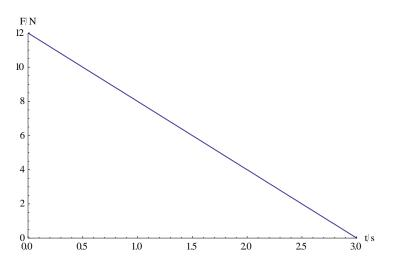
Method 1: The impulse is  $\frac{12 \times 3.0}{2} = 18 \text{ N s}$  and so the final speed is  $v = \frac{18}{2.0} = 9.0 \text{ m s}^{-1}$  The change in total energy is the change in kinetic energy  $\Delta E = \frac{1}{2} \times 2.0 \times 9.0^2 = 81 \text{ J}$  and dividing by the time to get
