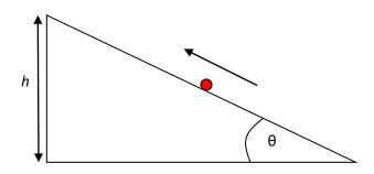
Method 1: The change in potential energy is  $mgh = 4.0 \times 10 \times 8.0 = 320$  J and this change occurs in a time of (the distance travelled along the plane is 16 m)  $t = \frac{16}{4.0} = 4.0$  s. There is no change in kinetic energy.
